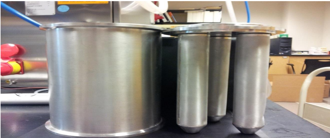
Figure 5.5 Fluidized Bed Filter House with Large Filters
