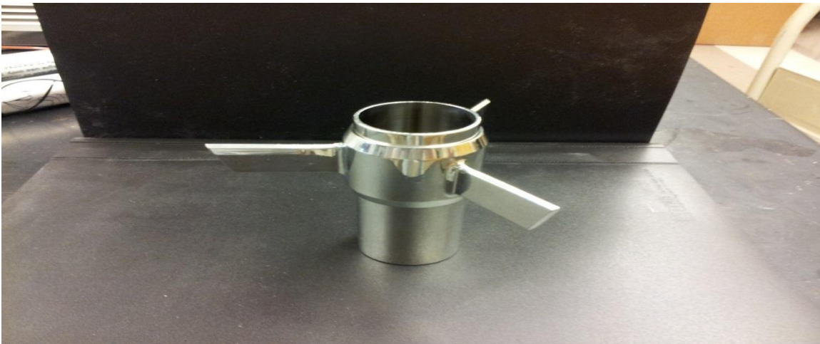
Figure 5.3 Fluidized Bed Wurster Insert
