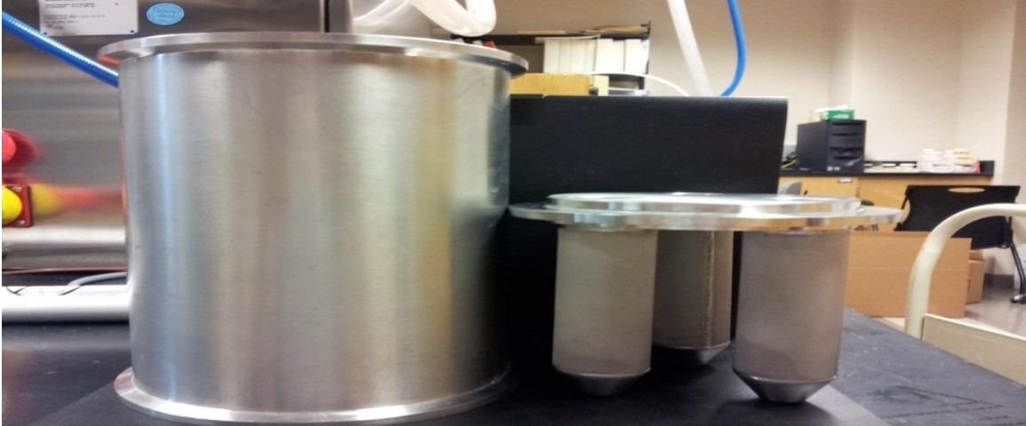
Figure 5.6 Fluidized Bed Filter House with Small Filters
