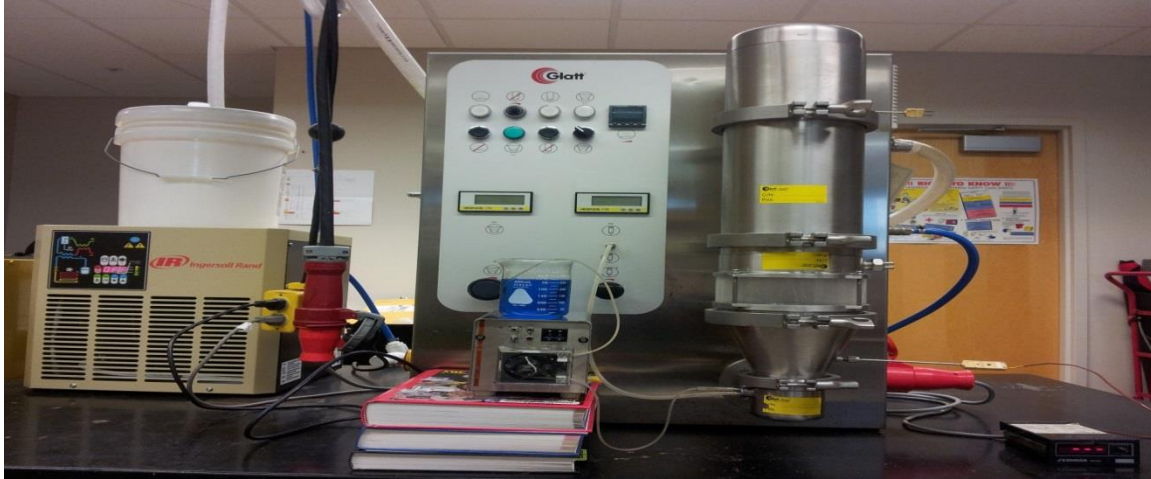
Figure 5.14 Fluidized Bed Completely Assembled in Wurster Orientation
