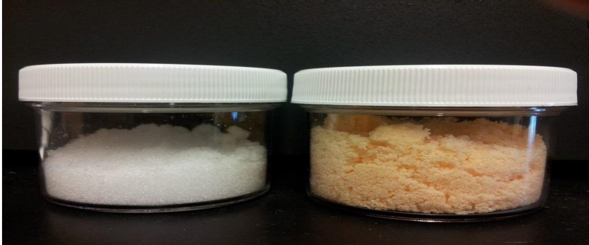
Figure 6.1 Ammonium Nitrate Particles Before (Left) and After (Right) a Coating Experiment
